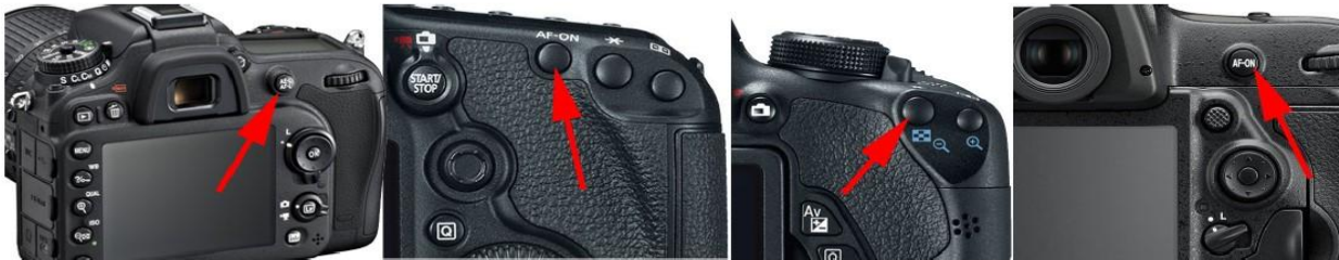
AF-On button options on Nikon and Canon cameras. NOTE - Most non-Rebel series Canon cameras will have a dedicated AF-On button, whereas only Nikon's higher end models have one, so you'll have to reassign the AE/AF lock button if AF-On is missing from yours.
